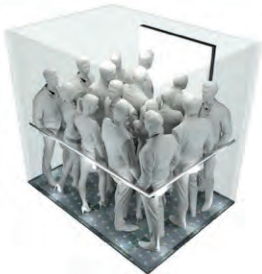
Figure 1: A 2000-kg/26-person elevator car holding 16 passengers; image courtesy of the British Council of Offices
